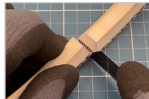
Carefully cut the coating of the belt
